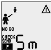
If your Barryvox® detects that the transmit frequency of the tested device is out of tolerance, a warning message will be shown. In this case, repeat the test with 5m distance between the participants to identify the defective transmitter. Such devices must be checked by the manufacturer.
