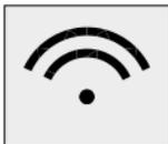
Each time the SEND mode is activated, this is confirmed by an ascending triple beep sound. Each individual signal pulse is tested. If the test is successful, this is confirmed by a blink of the red SEND-Control LED.
