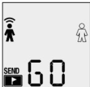
The test is successful if you can clearly hear beep sounds from each participant's transceiver within the range indicated on the display.
